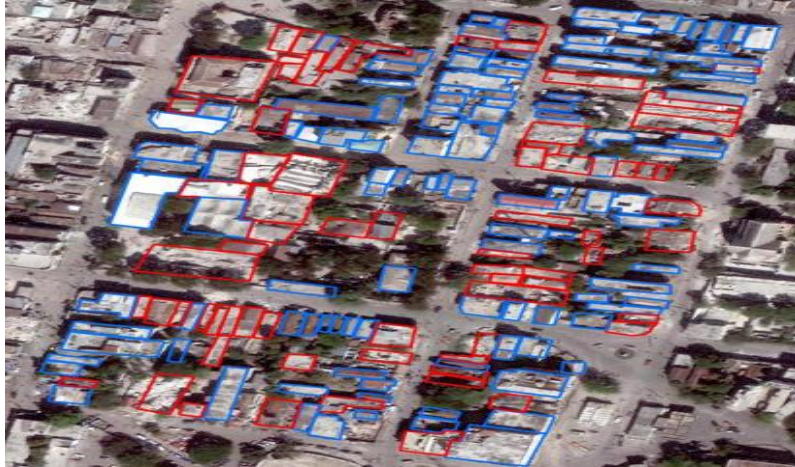
Fig.6. A test of sample B. Ones with damage are shown in red, whereas unharmed buildings are shown in blue.
